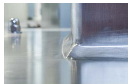
Weld seams ground free of cracks and gaps
